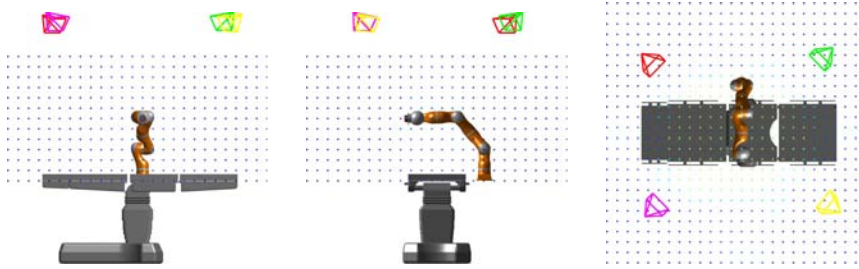
Figure 5.13.: Visualization of volume covered by at least one Kinect v1 camera from front, side and top perspective.
