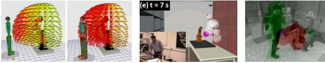
Figure 2.14.: Examples of (multi) 3D camera based concepts for safe human-robot collaboration. Left : Different risk estimation for robot poses based on viewing direction of user [26]; center : Approximation of user with spheres based on multi-camera skeleton tracking [126]; right : Intersection of danger zone around robot and safety zone around user based on occupancy grids [160].
