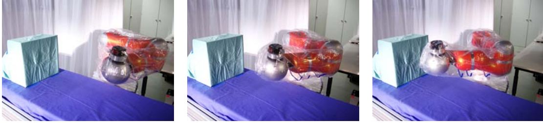
Figure 5.34.: Motion sequence performed by draped robot for evaluation of effects of surgical draping upon detection of impending collisions.
