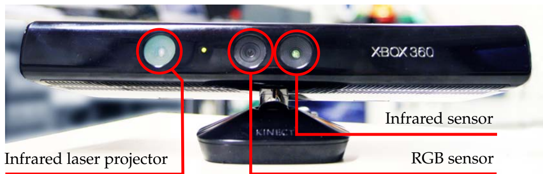
Figure 2.5.: Optical components of the Microsoft Kinect for Xbox 360.
