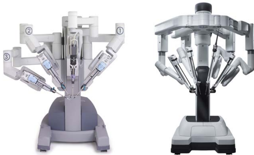
Figure 2.2.: Patient cart of the da Vinci™ with three arms for endoscopic instruments and one arm for the endoscopic camera. Left: da Vinci® Si™ (2009) [70], right: da Vinci® Xi™ (2014) [71]. ©2016 Intuitive Surgical, Inc.
