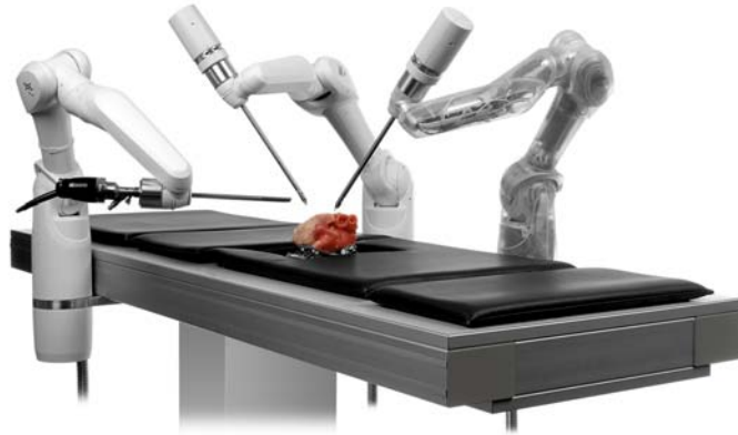
Figure 2.3.: The MiroSurge system with three lightweight MIRO arms that are directly attached to an OR table [37].
