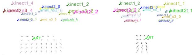
Figure 5.2.: Reconstructed origins of the coordinate system of different devices and locations of features that were projected on the surface of an OR table at five different heights, visualized from two different perspectives.
