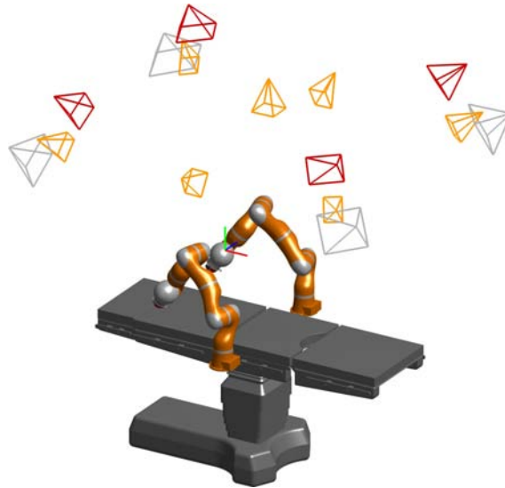
Figure 4.5.: Visualization of the camera poses relative to the OR table. Poses of PMD cameras are depicted in orange, Kinect v1 cameras in red and Kinect v2 cameras in gray. The coordinate system between both robots represents the origin of the optical tracking system ARTtrack2. Shapes of the camera pose markers represent the FoV of the corresponding camera.
